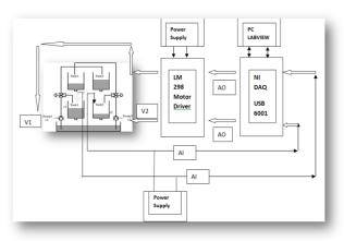
Figure: 2: Schematic Diagram of the Experimental Setup of QTS
