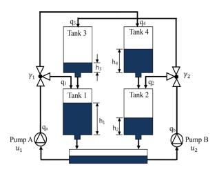
Figure: 1 Quadruple Tank System
